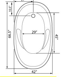
Some standard & most alternate pump locations may stickout past perimeter of the bath 1"-3". NOTE: Graphics may not be to scale. Specifications and features are subject to change without notice and are ± .25". All final measurements should be taken from tub on site. Access 18"x 18" or larger is required for each pump. Consult your contractor for installation requirements.
