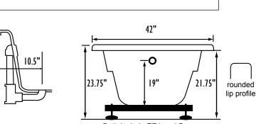
Bath include EZ Level Base INSTALLATION WILL NOT REQUIRE MORTAR BEDDING
