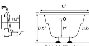
Bath include EZ Level Legs INSTALLATION WILL NOT REQUIRE MORTAR BEDDING
