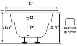
Bath include EZ Level Legs **INSTALLATION WILL NOT REQUIRE MORTAR BEDDING**
