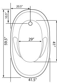
Some standard & most alternate pump locations may stickout past perimeter of the bath 1"-3". NOTE: Graphics may not be to scale.
