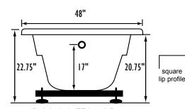
Bath include EZ Level Base **INSTALLATION WILL NOT REQUIRE MORTAR BEDDING**
