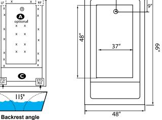
Some standard & most alternate pump locations may stickout past perimeter of the bath 1"-3". NOTE: Graphics may not be to scale. Specifications and features are subject to change without notice and are ± .25". All final measurements should be taken from tub on site. Access 18"x 18" or larger is required for each pump. Consult your contractor for installation requirements.
