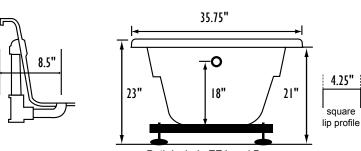
Bath include EZ Level Base INSTALLATION WILL NOT REQUIRE MORTAR BEDDING
