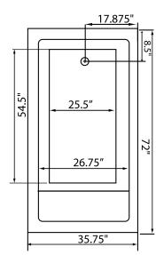
Some standard & most alternate pump locations may stickout past perimeter of the bath 1"-3". NOTE: Graphics may not be to scale. Specifications and features are subject to change without notice and are ± .25". All final measurements should be taken from tub on site. Access 18"x 18" or larger is required for each pump. Consult your contractor for installation requirements.
