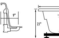
Bath include EZ Level Base **INSTALLATION WILL NOT REQUIRE MORTAR BEDDING**
