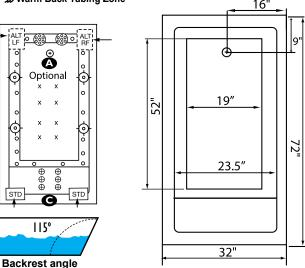
Some standard & most alternate pump locations may stickout past perimeter of the bath 1"-3". NOTE: Graphics may not be to scale. Specifications and features are subject to change without notice and are ± .25". All final measurements should be taken from tub on site.
