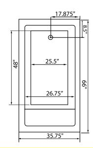
Some standard & most alternate pump locations may stickout past perimeter of the bath 1"-3". NOTE: Graphics may not be to scale.
