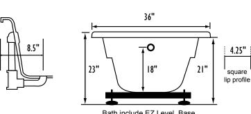
Bath include EZ Level Base **INSTALLATION WILL NOT REQUIRE MORTAR BEDDING**
