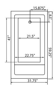
Some standard & most alternate pump locations may stickout past perimeter of the bath 1"-3". NOTE: Graphics may not be to scale. Specifications and features are subject to change without notice and are ± .25". All final measurements should be taken from tub on site.
