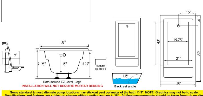
Some standard & most alternate pump locations may stickout past perimeter of the bath 1"-3". NOTE: Graphics may not be to scale. Specifications and features are subject to change without notice and are ± .25". All final measurements should be taken from tub on site. Access 18"x 18" or larger is required for each pump. Consult your contractor for installation requirements.
