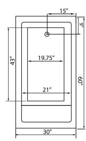
Some standard & most alternate pump locations may stickout past perimeter of the bath 1"-3". NOTE: Graphics may not be to scale.
