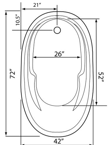
Some standard & most alternate pump locations may stickout past perimeter of the bath 1"-3". NOTE: Graphics may not be to scale. Specifications and features are subject to change without notice and are  $\pm .25"$ . All final measurements should be taken from tub on site. Access 18"x 18" or larger is required for each pump. Consult your contractor for installation requirements.
