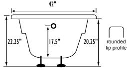
Bath include EZ Level Legs INSTALLATION WILL NOT REQUIRE MORTAR BEDDING
