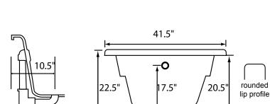
Bath include EZ Level Base **INSTALLATION WILL NOT REQUIRE MORTAR BEDDING**
