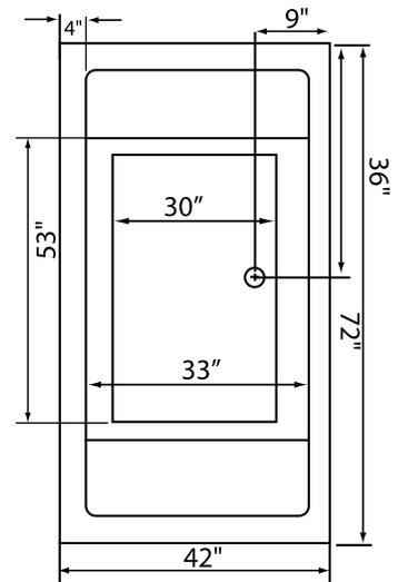
**NOTE:** Graphics may not be to scale. Specifications and features are subject to change without notice and are  $\pm .25"$ . All final measurements should be taken from **tub on site**. Access 18"x 18" or larger is required for each pump. Some pump locations and plumbing may extend beyond the perimeter of the bath.
