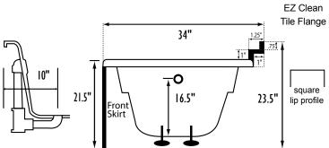
Bath includes EZ Level Legs **INSTALLATION WILL NOT REQUIRE MORTAR BEDDING**
