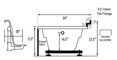
Bath includes EZ Level Base INSTALLATION WILL NOT REQUIRE MORTAR BEDDING
