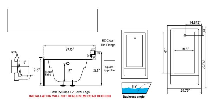
**NOTE:** Graphics may not be to scale. Specifications and features are subject to change without notice and are ± .25". All final measurements should be taken from **tub on site.** Access 18"x 18" or larger is required for each pump. Some pump locations and plumbing may extend beyond the perimeter of the bath.
