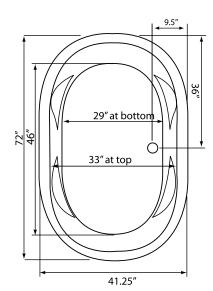
Some standard & most alternate pump locations may stickout past perimeter of the bath 1"-3". NOTE: Graphics may not be to scale. Specifications and features are subject to change without notice and are ± .25". All final measurements should be taken from tub on site.
