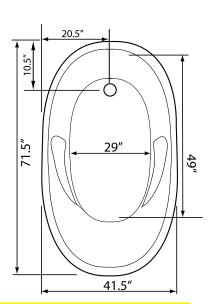
Bath include EZ Level Legs INSTALLATION WILL NOT REQUIRE MORTAR BEDDING
