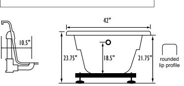
Bath include EZ Level Base INSTALLATION WILL NOT REQUIRE MORTAR BEDDING
