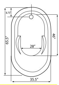
Some standard & most alternate pump locations may stickout past perimeter of the bath 1"-3". NOTE: Graphics may not be to scale. Specifications and features are subject to change without notice and are ± .25". All final measurements should be taken from tub on site. Access 18"x 18" or larger is required for each pump. Consult your contractor for installation requirements.
