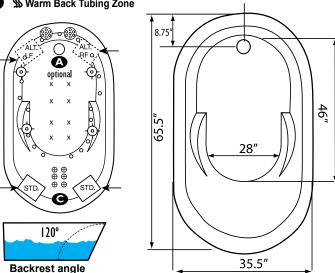
Some standard & most alternate pump locations may stickout past perimeter of the bath 1"-3". NOTE: Graphics may not be to scale. Specifications and features are subject to change without notice and are ± .25". All final measurements should be taken from tub on site. Access 18"x 18" or larger is required for each pump. Consult your contractor for installation requirements.
