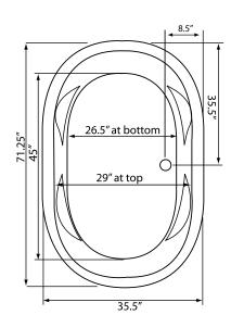
Some standard & most alternate pump locations may stickout past perimeter of the bath 1"-3". NOTE: Graphics may not be to scale.
