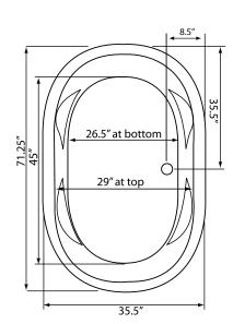
Some standard & most alternate pump locations may stickout past perimeter of the bath 1"-3". NOTE: Graphics may not be to scale. Specifications and features are subject to change without notice and are ± .25". All final measurements should be taken from tub on site.
