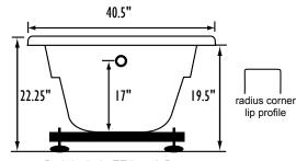
Bath include EZ Level Base **INSTALLATION WILL NOT REQUIRE MORTAR BEDDING**
