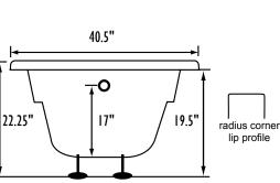
Bath include EZ Level Legs **INSTALLATION WILL NOT REQUIRE MORTAR BEDDING**
