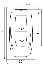
Some standard & most alternate pump locations may stickout past perimeter of the bath 1"-3". NOTE: Graphics may not be to scale.
