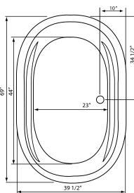
NOTE: Graphics may not be to scale. Specifications and features are subject to change without notice and are ± .25". All final measurements should be taken from tub on site. Access 18"x 18" or larger is required for each pump. Some pump locations and plumbing may extend beyond the perimeter of the bath.
