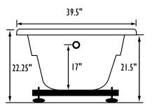
Bath includes EZ Level Base **INSTALLATION WILL NOT REQUIRE MORTAR BEDDING**
