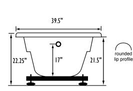
Bath includes EZ Level Base **INSTALLATION WILL NOT REQUIRE MORTAR BEDDING**
