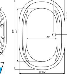
NOTE: Graphics may not be to scale. Specifications and features are subject to change without notice and are ± .25". All final measurements should be taken from tub on site. Access 18"x 18" or larger is required for each pump. Some pump locations and plumbing may extend beyond the perimeter of the bath.
