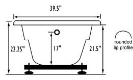
Bath includes EZ Level Base **INSTALLATION WILL NOT REQUIRE MORTAR BEDDING**
