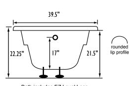
Bath includes EZ Level Legs **INSTALLATION WILL NOT REQUIRE MORTAR BEDDING**  A X HTT® Leg Therapy Air Massage System includes 10 Air Jets on the floor. Optional on Combo Plat and Combo Gold Series B X 6 Jet HTT® Back Massage System: N/A on Combo Series-Standard on Plat series **ⓒ SS** Warm Back Tubing Zone
