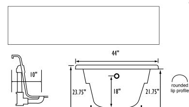
Bath includes F7 Level Base INSTALLATION WILL NOT REQUIRE MORTAR BEDDING
