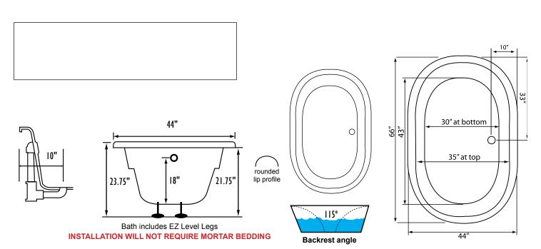
Some standard & most alternate pump locations may stickout past perimeter of the bath 1"-3". NOTE: Graphics may not be to scale. Specifications and features are subject to change without notice and are ± .25". All final measurements should be taken from tub on site. Access 18"x 18" or larger is required for each pump. Consult your contractor for installation requirements.
