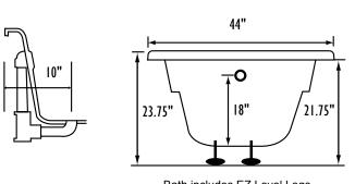
Bath includes EZ Level Legs **INSTALLATION WILL NOT REQUIRE MORTAR BEDDING**
