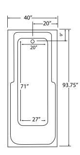
NOTE: Graphics may not be to scale. Specifications and features are subject to change without notice and are ± .25". All final measurements should be taken from tub on site. Access 18"x 18" or larger is required for each pump. Some pump locations and plumbing may extend beyond the perimeter of the bath.
