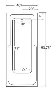
NOTE: Graphics may not be to scale. Specifications and features are subject to change without notice and are ± .25". All final measurements should be taken from tub on site. Access 18"x 18" or larger is required for each pump. Some pump locations and plumbing may extend beyond the perimeter of the bath.
