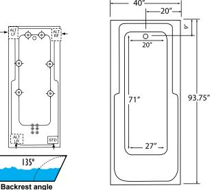
NOTE: Graphics may not be to scale. Specifications and features are subject to change without notice and are ± .25". All final measurements should be taken from tub on site. Access 18"x 18" or larger is required for each pump. Some pump locations and plumbing may extend beyond the perimeter of the bath.
