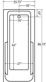
Bath include EZ Level Legs **INSTALLATION WILL NOT REQUIRE MORTAR BEDDING**
