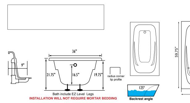
**NOTE:** Graphics may not be to scale. Specifications and features are subject to change without notice and are ± .25". All final measurements should be taken from **tub on site.** Access 18"x 18" or larger is required for each pump. Some pump locations and plumbing may extend beyond the perimeter of the bath.
