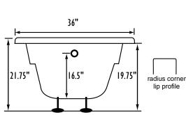
Bath include EZ Level Legs **INSTALLATION WILL NOT REQUIRE MORTAR BEDDING**  **ⓒ SWarm Back Tubing Zone** A
