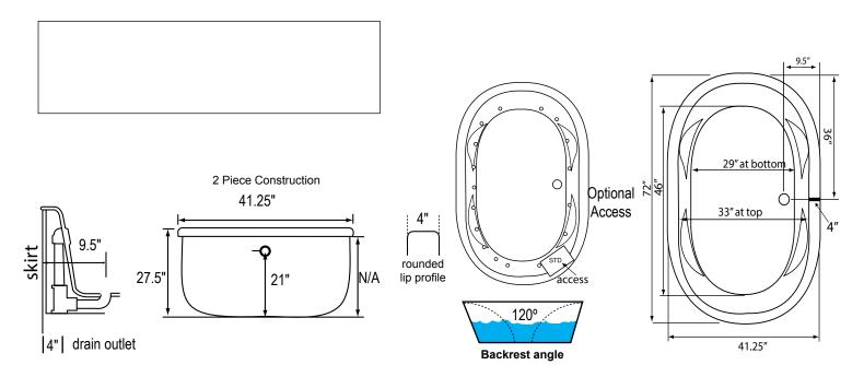
Some standard & most alternate pump locations may stickout past perimeter of the bath 1"-3". NOTE: Graphics may not be to scale. Specifications and features are subject to change without notice and are ± .25". All final measurements should be taken from tub on site.
