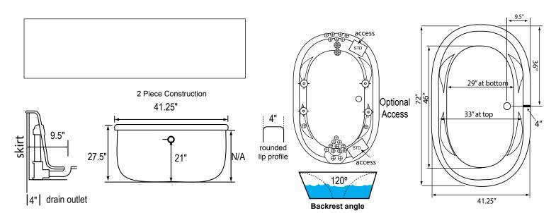
Some standard & most alternate pump locations may stickout past perimeter of the bath 1"-3". NOTE: Graphics may not be to scale. Specifications and features are subject to change without notice and are ± .25". All final measurements should be taken from tub on site.
