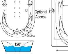
Some standard & most alternate pump locations may stickout past perimeter of the bath 1"-3". NOTE: Graphics may not be to scale. Specifications and features are subject to change without notice and are ± .25". All final measurements should be taken from tub on site. Access 18"x 18" or larger is required for each pump. Consult your contractor for installation requirements.
