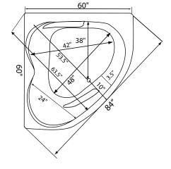
NOTE: Graphics may not be to scale. Specifications and features are subject to change without notice and are ± .25". All final measurements should be taken from tub on site. Access 18"x 18" or larger is required for each pump. Some pump locations and plumbing may extend beyond the perimeter of the bath.
