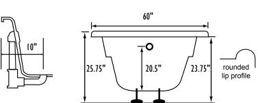
Bath includes EZ Level Legs **INSTALLATION WILL NOT REQUIRE MORTAR BEDDING**
